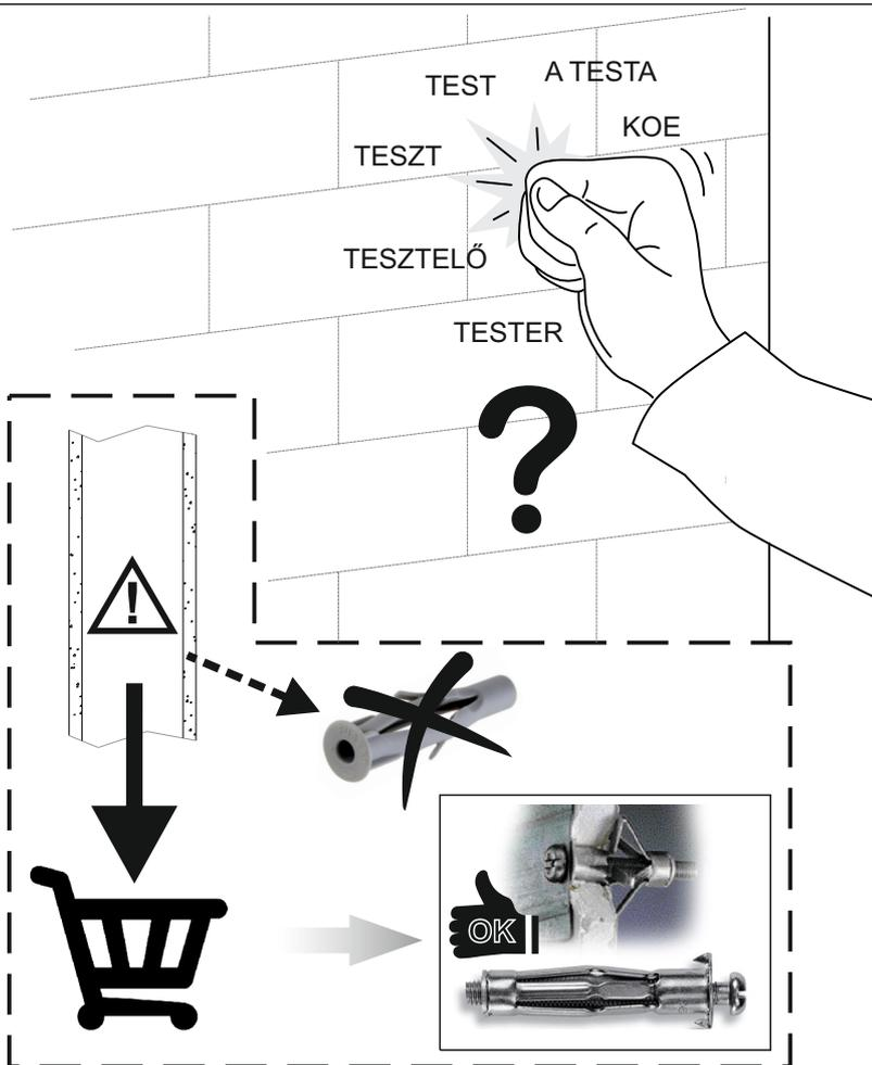
**(EN)** Caution! The wall must be examined before assembly. The included universal wall plugs are only suitable for use on solid masonry such as concrete blocks or solid bricks or hollow bricks. Do not use these wall plugs on lightweight block masonry, surfaces such as drywall or framed walls. In these cases, use specific special plugs! These can be purchased in a dedicated shop (hardware store). In case of non-compliance, the manufacturer/retailer or the importer assumes no responsibility.
